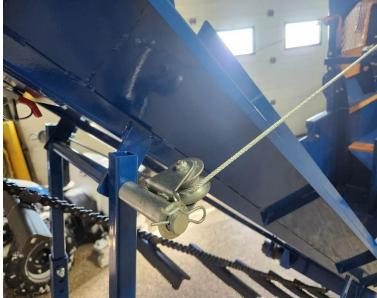
Install the rod with the winch pulleys AND the support leg onto the lower section of the conveyor. Run the cable back around the conveyor and hook it onto the left side of the tower on the machine.
