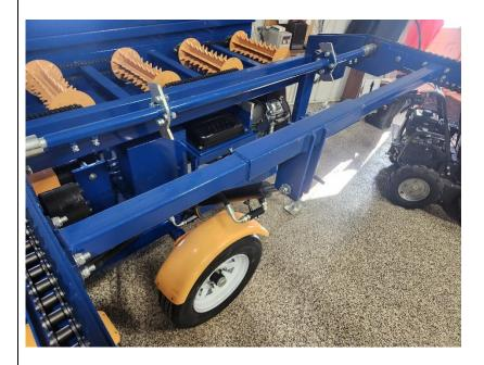
Install cylinder support bar between tables side and install lifting cylinder on support bar/ frame of machine.
