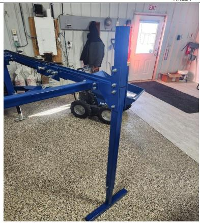
Install end legs onto each side of the table - uprights can be installed at this time too.
