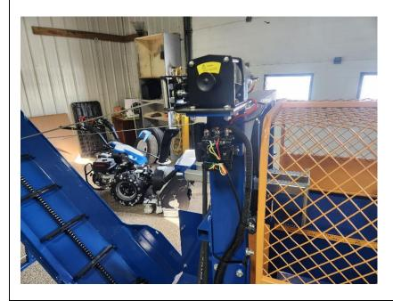
The lifting cylinder can now be mounted to the splitting wedge via two small, blue flat-bar brackets and the provided bolts.
