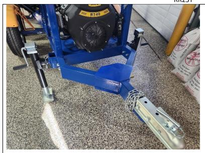
Install draw bar assembly with coupler and safety chains.
