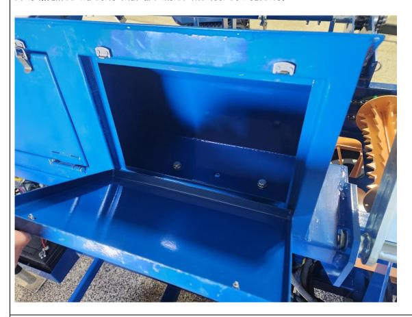
Place the splitting wedge into its pocket at the rear of the machine. For now - it will set all the way down - it will be attached to the lifting cylinder in a later step.
