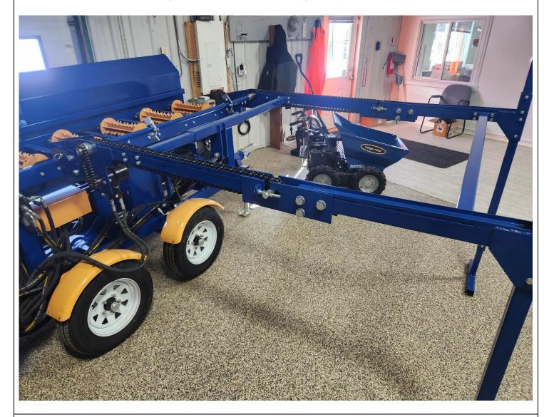
Build the table sides separately, on the ground. Once they are both assembled, one side will be installed onto the machine at a time.
