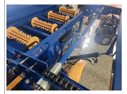
Install both sides of table to frame of machine - then install blue bar with silver ends(chain drive bar)
