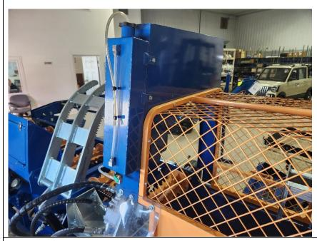
The cage/guard assembly can then be mounted to the frame of the machine via the long mounting pin – it has cotter pins and washer on both ends to lock it in place.
