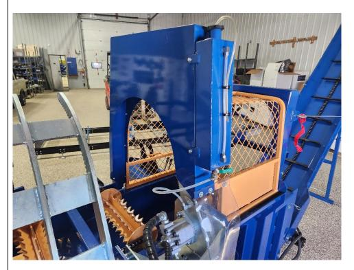
Attach the orange cage to the blue saw guard via the bolts in the cage, don't tighten these bolts fully just yet.
