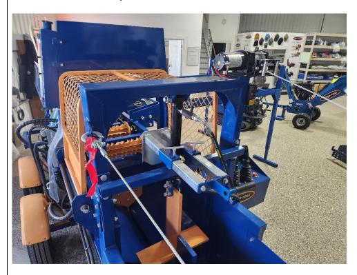
Locate the "U"- shaped tower and install it on the back of the machine using the bolts provided.
